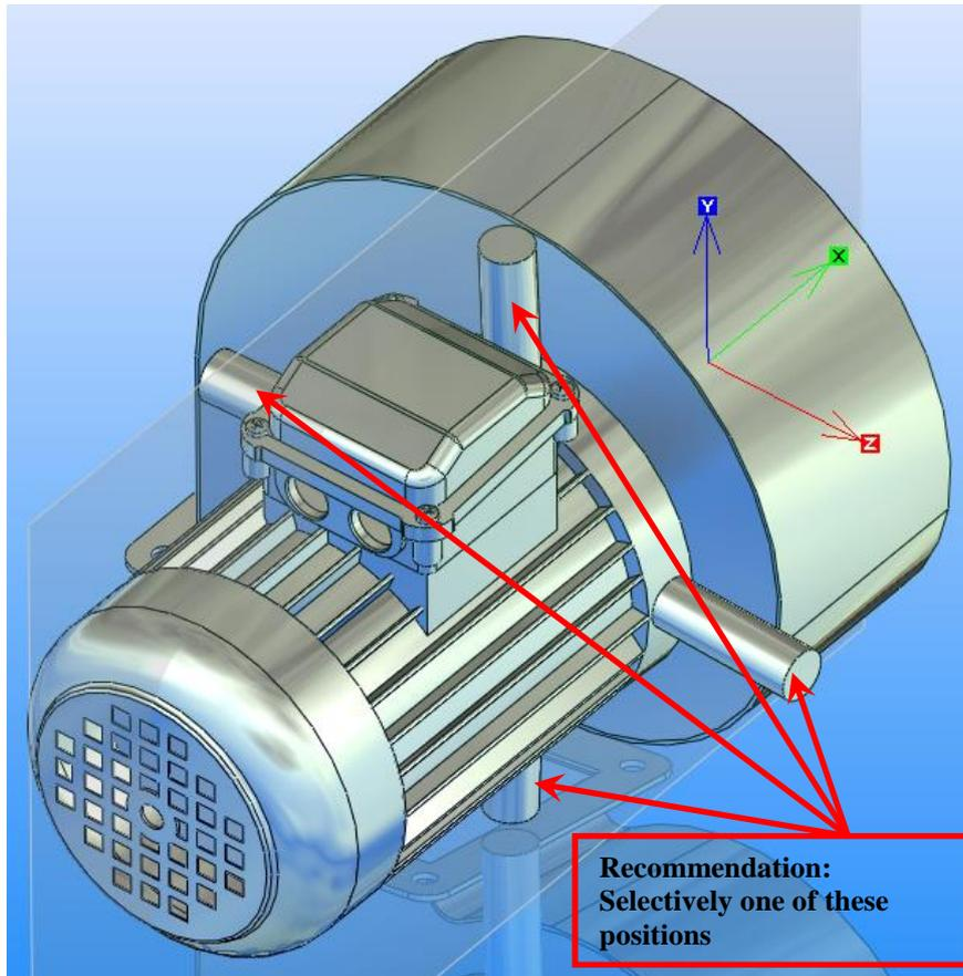
**Scheme illustration: Recommendations for positioning of vibration sensor**
